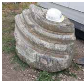
Figure 7. Large Boulder Pushed by MTBM
