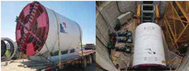
Figure 2. Custom Manufactured MTBM
