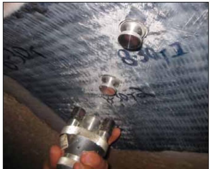
Figure 4 – Pull-off testing of the CFRP material within selected pipe section.
