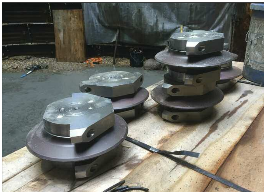
Figure 2. Replacement disc cutters
