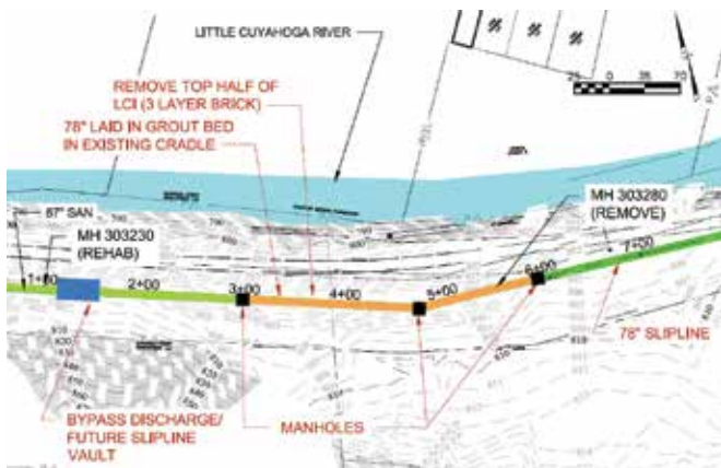
Figure 5 – Same Trench Replacement at Sag
