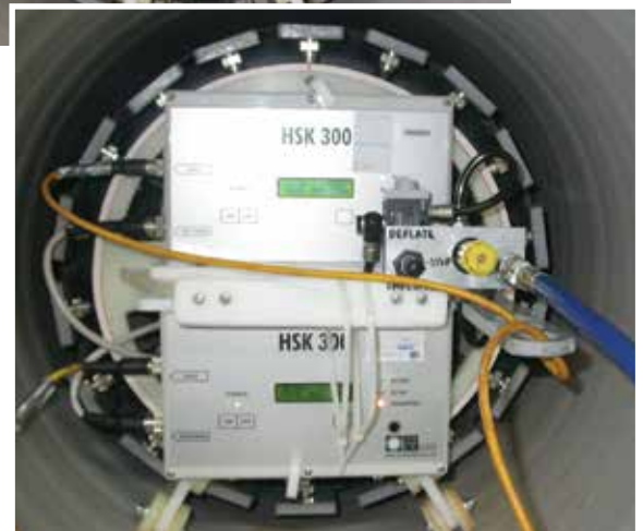
The PIG (Pipe Inspection Gauge) moves through the pipes via tether or rod and takes three readings per section. It can handle up to 90 degree bends with a single point of entry
