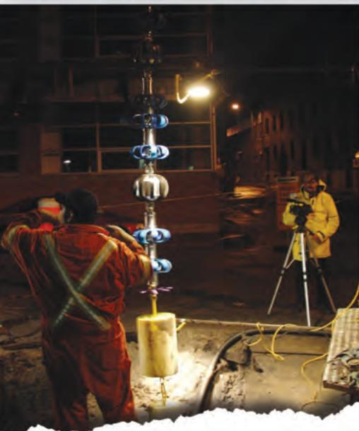
PICA helps Asset Managers who are serious about managing their pipeline assets proactively and fixing leaks before they can actually happen. With PICA's set of non-destructive testing tools, Asset Managers can know the real condition of their buried pipelines. Good information is powerful: pipelines can be surgically repaired, rehabilitated with liners, or partially replaced, thus extending their useful life while at the same time reducing risk of failure (and sleepless nights).
