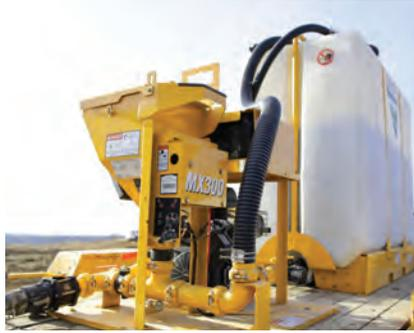
The right-sized mixing system is key for drilling operations. With a redesigned, slim rectangular profile tank, the new Vermeer MX300 mixing system helps horizontal directional drilling (HDD) contractors optimize productivity and offers customizable mounting configuration options.
