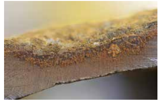
Graphitization cross section
