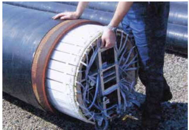
Internal pig probe with multiple sensors
