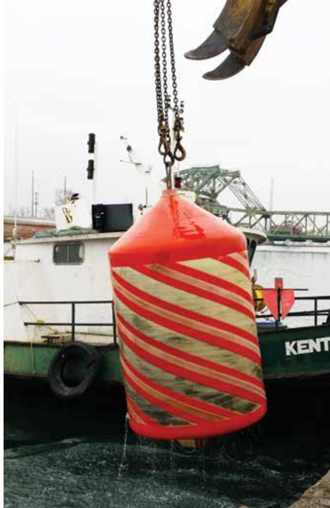
Figure 6.60-inch brush pig after being towed to shore
