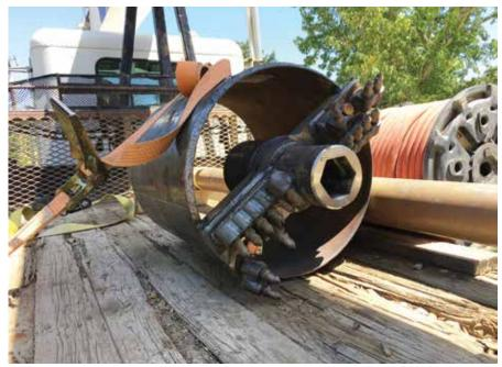
Auger head with bullet teeth to excavate in hard ground
