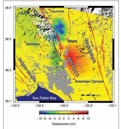
Figure 2: Ground Deformation from the South Napa Earthquake
