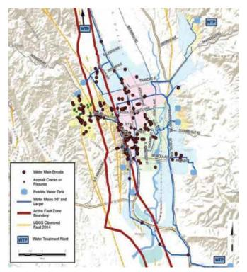
Figure 4: Earthquake Caused Water Pipeline Leaks
