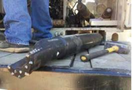
Bits are now available for guided boring machines that excavate during the pilot phase
