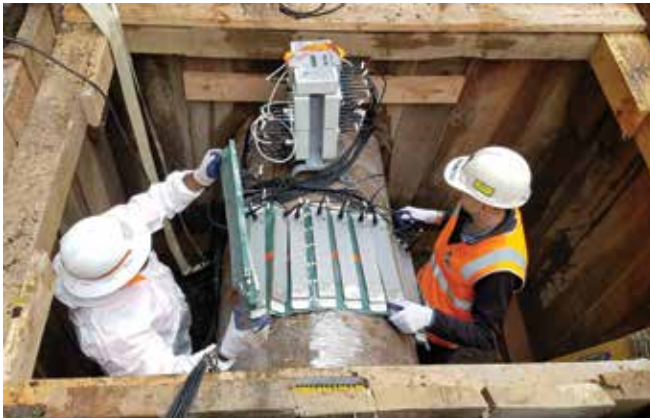
The Flexible Array Scanning Tool (FAST) strips adjust to the pipe circumference and form a “blanket.” Inside each strip are sensors, antennae and cables that connect to the core processor
