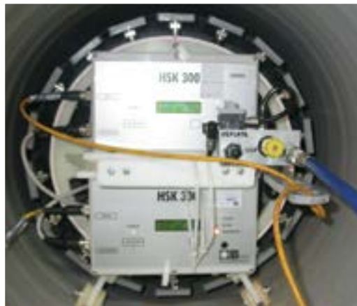
The PIG (Pipe Inspection Gauge) moves through the pipes via tether or rod and takes three readings per section. It can handle up to 90 degree bends with a single point of entry
