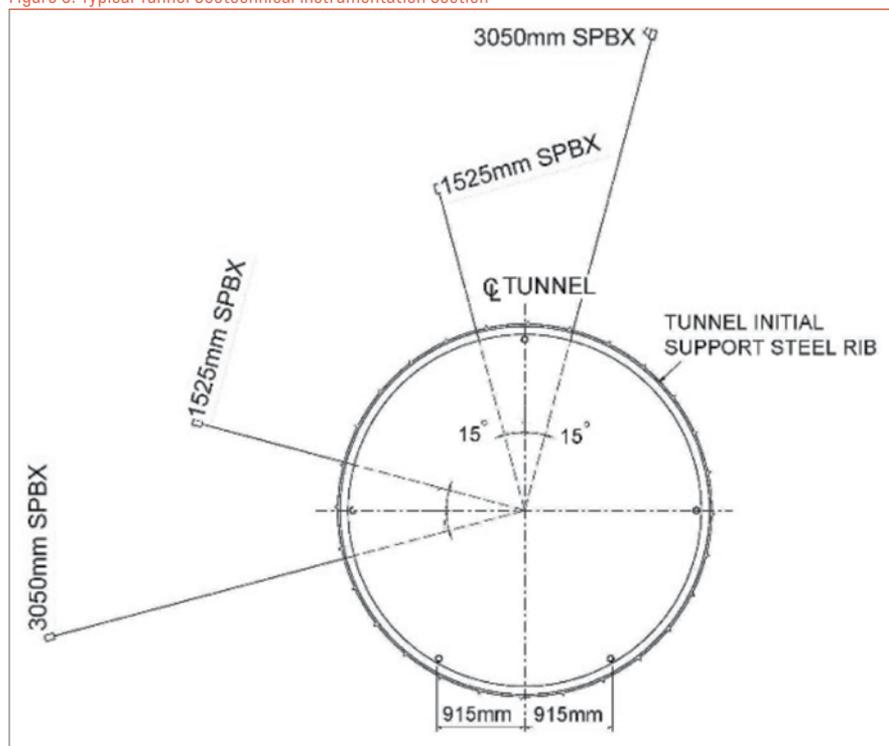
instrumentation section for the tunnel.
