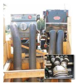
Maintaining a minimum 45mph velocity was an achievement, considering pipe diameter and geometry
