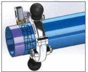
Scrape or peel the pipe to remove the surface layer and expose clean virgin pipe beneath
