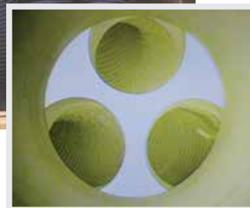
Dust collector with three 16-inch hoses was used to recover leftover cleaning grit
