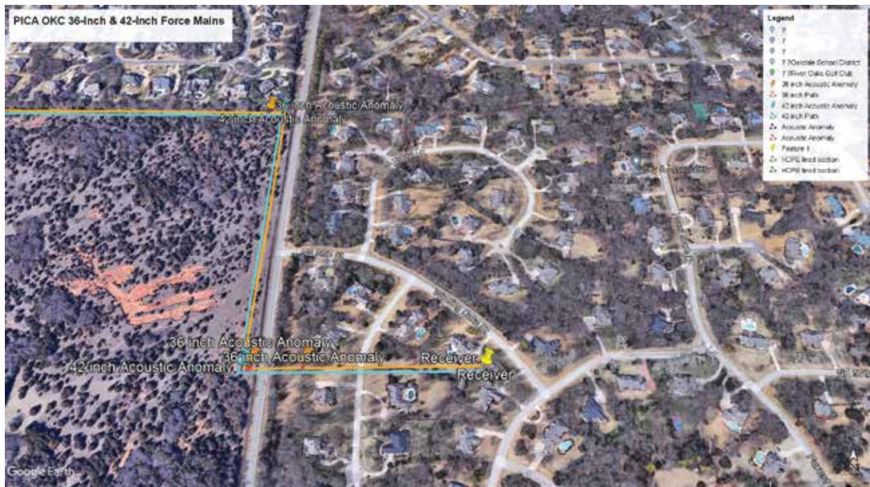
Figure 4. Zoom of the pipeline section of the 36-inch and 42-inch force mains with the acoustic anomalies. Based on the locations and confirmation of the air-pockets OKCWUT will perform external validations utilizing the PICA Bracelet Probe (Figure 2) to identify the wall loss in these areas and determine the RUL (Remaining Useful Life) of this critical asset
