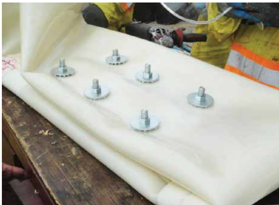
Liner with six tail bolts
