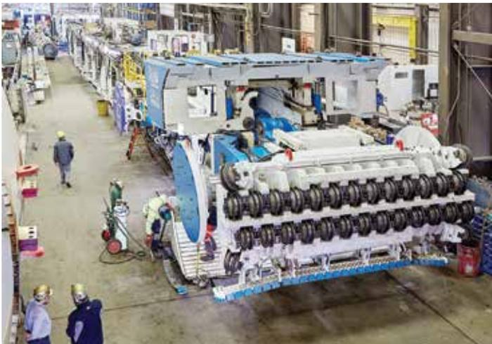
*The MDM5000 (standing for Mine Development Machine with dimensions of 5.0 m x 4.5 m) is capable of excavating a flat tunnel invert in hard rock.*
