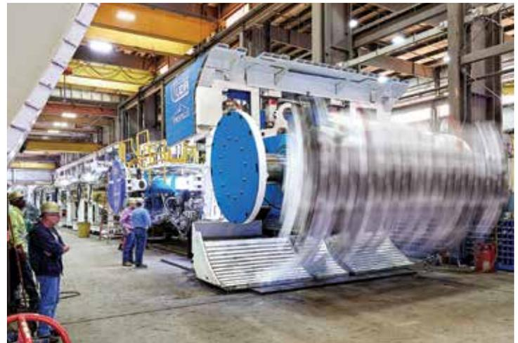
*Developed by Robbins for use in rock up to 200 MPa UCS, the MDM5000 excavates with a reciprocating cutterhead and swinging cutterhead motion to create a rectangular cross section tunnel.*
