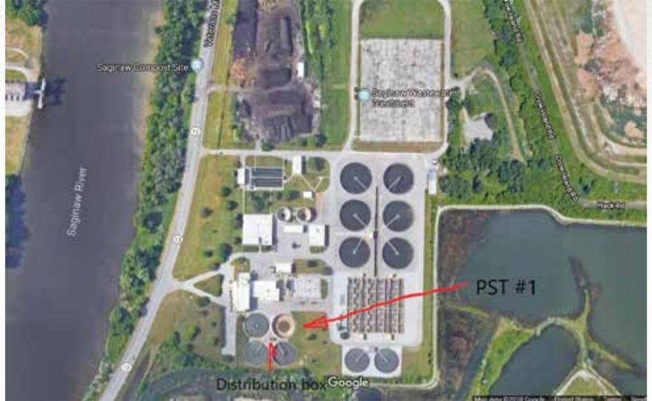
Figure 1. Saginaw WWTP with PST #1 and the distribution box identified
