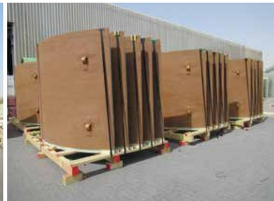
Proprietary system offered a way to break the geometrically complex pipe liners down into multiple component segments to dramatically reduce shipping costs, while still maintaining structural integrity and load capacity
