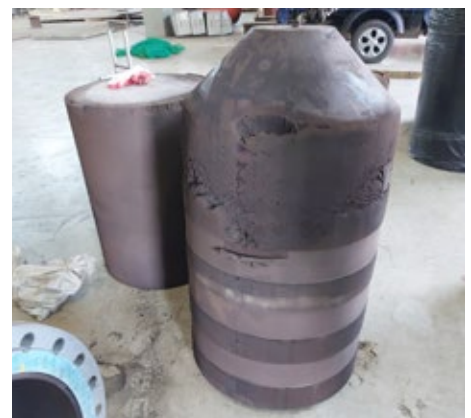
Figure 2: Foam pigs used for displacing liquid
