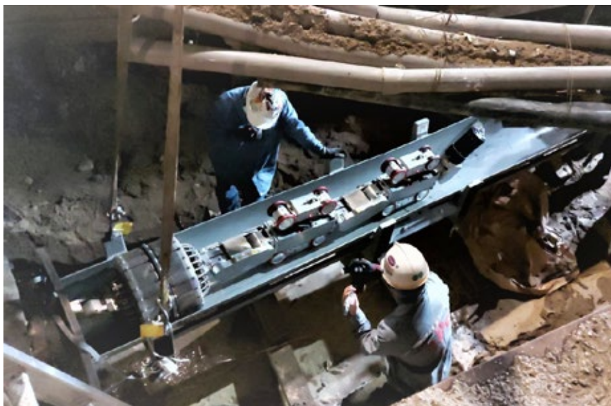
Figure 4: The Pipe Explorer being aligned to the 24-inch pipe
