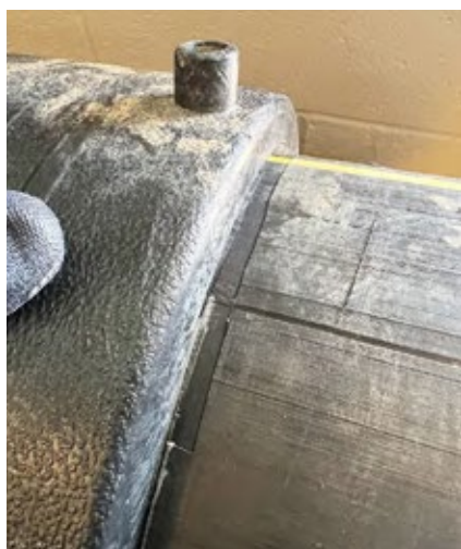
EF Fitting with suspected Bentonite contamination and severe gouge
