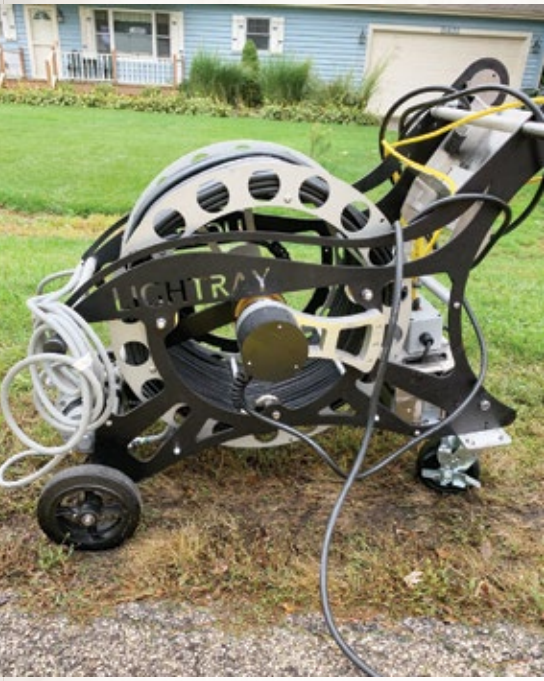
Figure 6. The LightRay LED UV light system for curing the T-Liner
