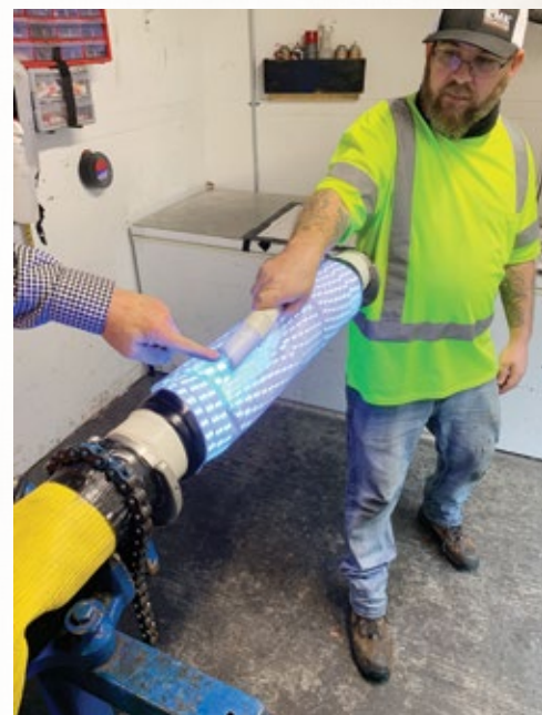
Figure 5. Double Strand LED UV Light Train
