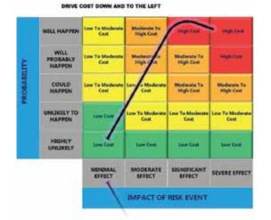
Figure 1 – Driving risk down. The intent of risk-based engineering is to drive cost down from red to orange to yellow to green by driving risk down to more manageable levels.
