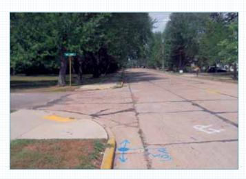
Figure 1 – Palmetto Avenue where it is intersected by Wallonnie Drive. The pipe varies in location from under the curb to near the middle of the lane in the foreground. Excavation would disturb much of the pavement.
