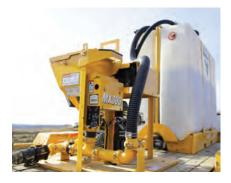
The right-sized mixing system is key for drilling operations. With a redesigned, slim rectangular profile tank, the new Vermeer MX300 mixing system helps horizontal directional drilling (HDD) contractors optimize productivity and offers customizable mounting configuration options.
