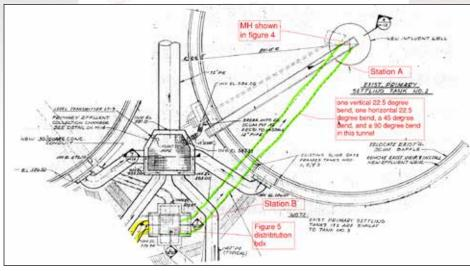
Figure 7. Plan view of PST#1 influent conduit
