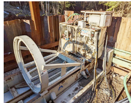
Akkerman Model 5000 Series II Pump System delivers up to 400 tons of jacking force
