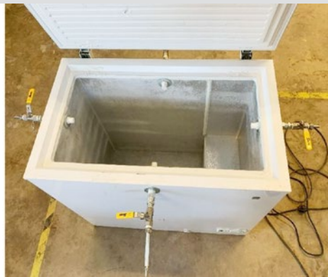
Secure testing chamber that represents the refrigerated transport truck is shown
