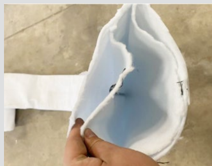
Two examples of uncured liners are shown
