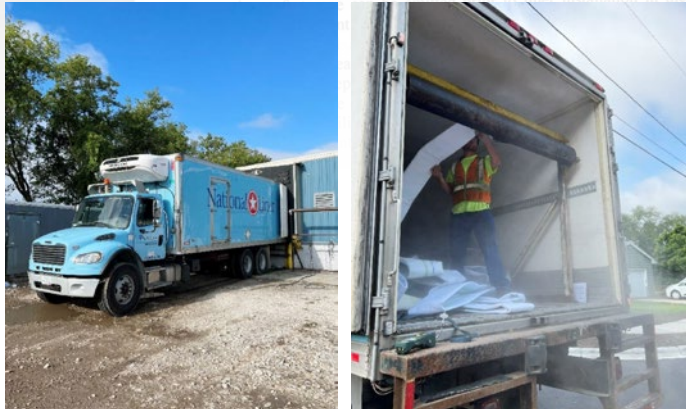
The "Reefer" or refrigerated truck used for wetted out liner transportation
