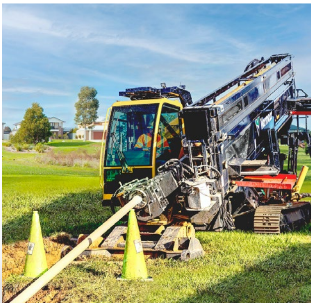
Large HDD rigs with onboard cab and rod rack are ideal for urban areas with limited space
