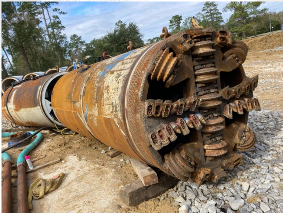
Figure 5. Akkerman SL60 MTBM
