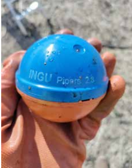
Figure 1: In-Line Screening Pipers® Device
