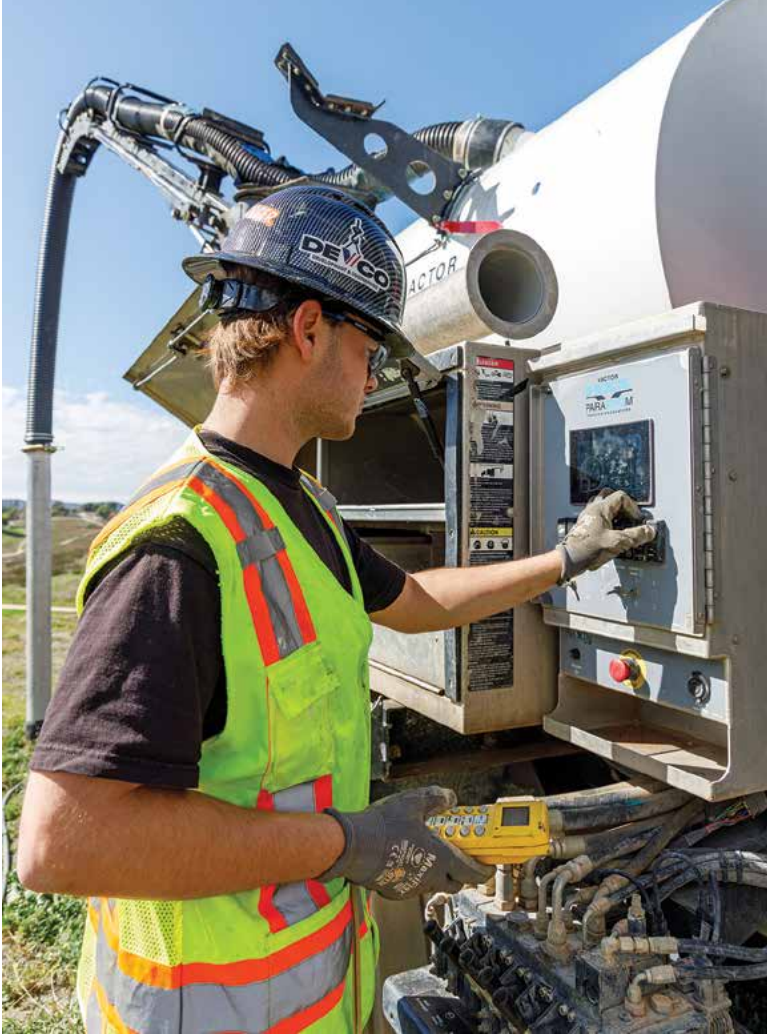
Drake Rossi sets up the HXX Paradigm (TRUVAC) hydroexcavator on a job site in Temecula, California. Hydroexcavation and HDD work are the mainstay of the company's business.
