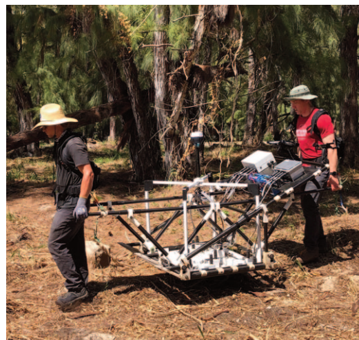
Figure 5. APEX operation in the chariot mode (left) and hand-carry mode (right) using the hand-carry attachment
