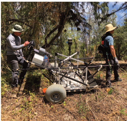
Figure 5. APEX operation in the chariot mode (left) and hand-carry mode (right) using the hand-carry attachment
