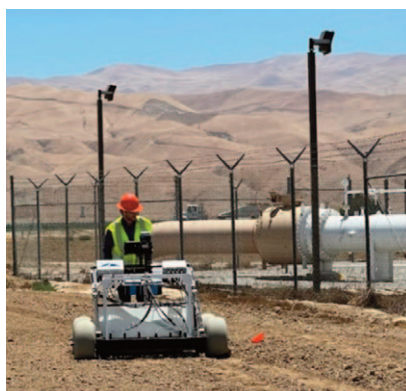
Figure 1. Operation of WRT APEX for detecting an underground transmission pipeline survey during a pilot demonstration in Wheeler Ridge, CA
