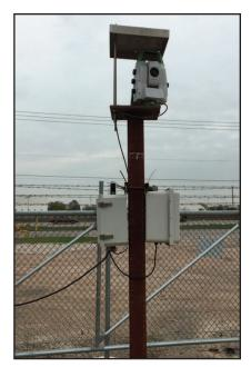
Figure 5. Survey monitors were used for a detailed surface settlement monitoring program
