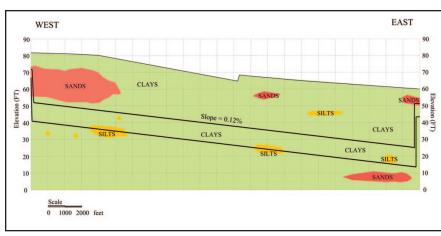
Figure 2. Segment B3 Tunnel horizon ground conditions were predominantly clays, with minor sand and silt lenses
