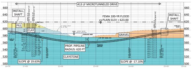
Figure 3. Guadalupe River crossing profile (1H:1V scale) with ground conditions shown (southwest bank is on left)
