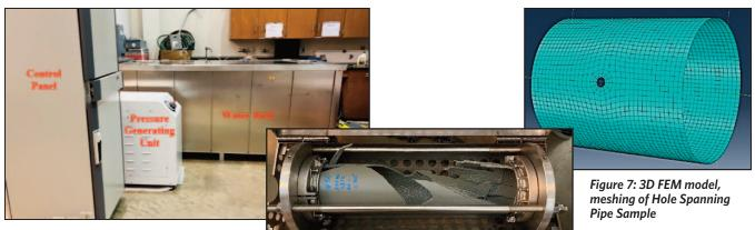
Figure 5: Hydrostatic Pressure Testing Equipment
