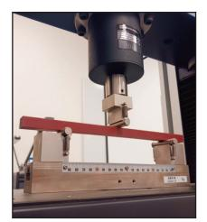
Figure 2: Short-term Flexural Testing
