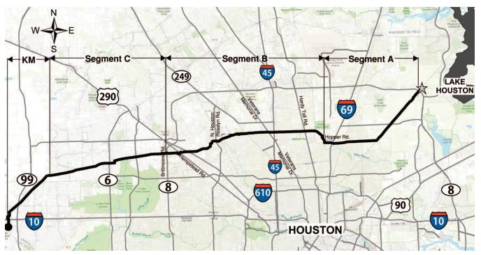
Figure 1. Surface Water Supply Project Alignment Map - approximately 42 miles of welded steel potable water pipelines
