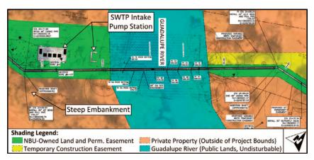
Figure 2. SWTP Discharge Water Line Guadalupe River crossing alignment
