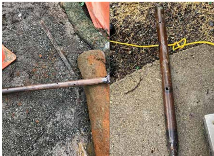
Figure 13. Grout shoes used to allow grout into the borehole
