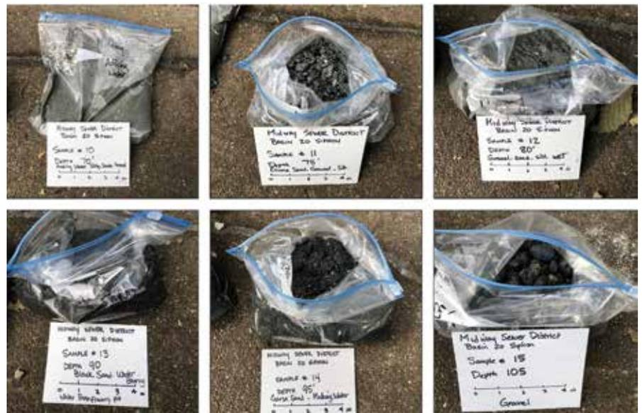
Figure 9. Soil samples from well drilled into pressurized aquifer (70’ to 105’ (21.3 m to 32 m) depth)
