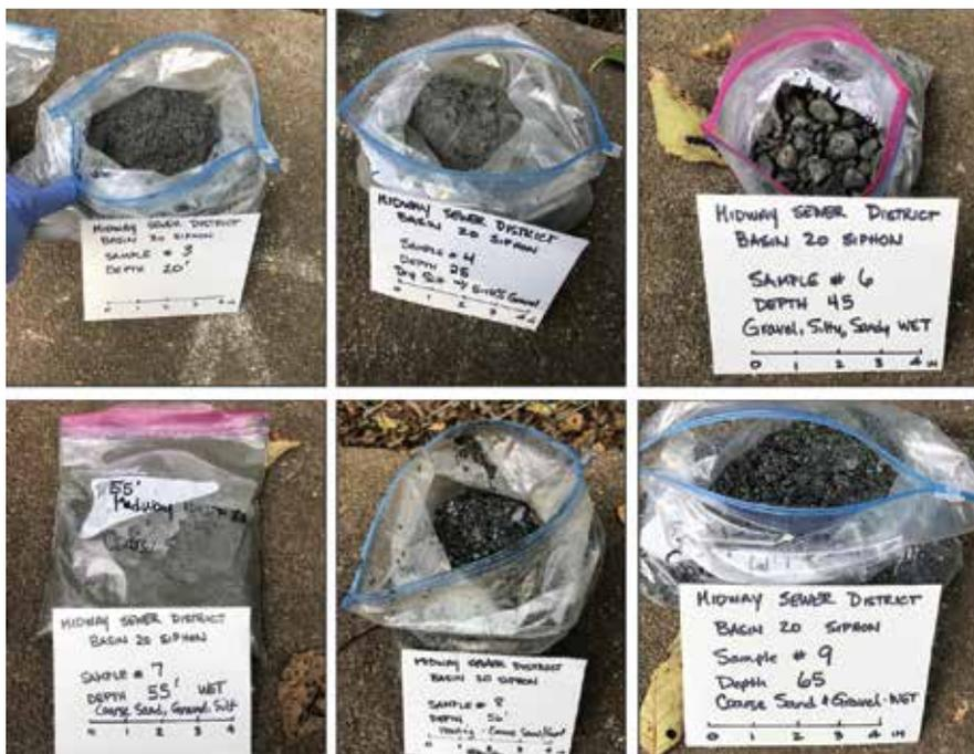
Figure 8. Soil samples from well drilled into pressurized aquifer (20' to 65' (6.1 m to 19.9 m) depth)
