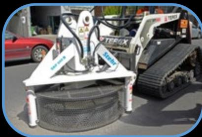
*Protective Liner Systems is a distributor for Stehr manhole cutters.*
