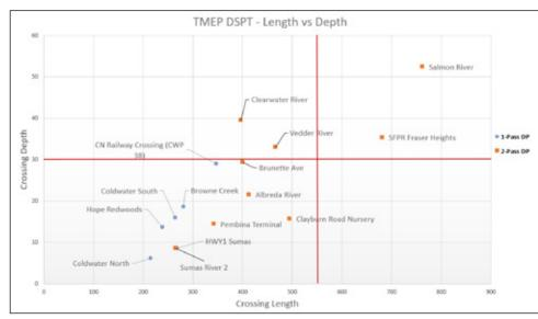
Figure 7. Trans Mountain Direct Pipe Crossings Length vs Depth
