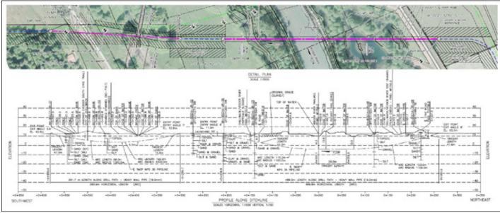
Figure 10. Back to back Direct Pipe Crossings
