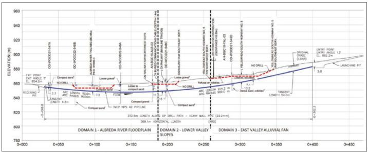
Figure 8. Albreda NPS 42 Triple Crossing of River/Highway/Railway
