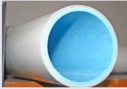
Finished CIPP liner inside PVC pipe
