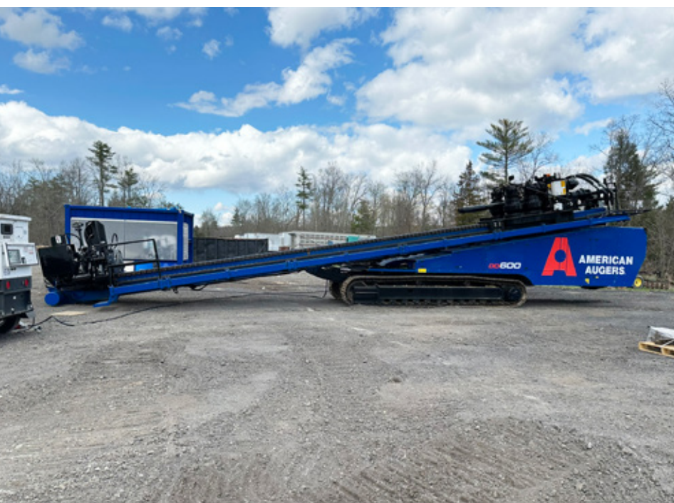
Figure 2: Drill Rig - 600,000 pounds of force
