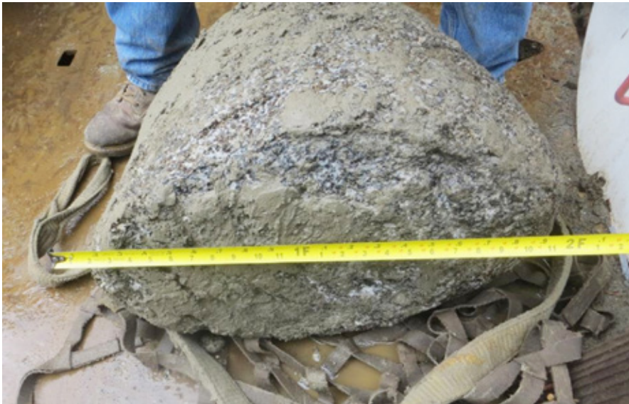
Figure 6 Boulder that was recovered from machine face. Note the tape measure is for scale. The largest dimension was measured with calipers that could measure up to 36-inches
