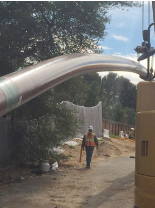
Figure 2. Plastic Bending of Steel Pipe at the Failure Radius
