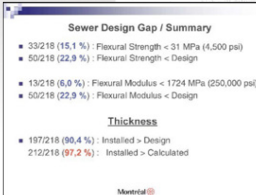
Figure 2. Summary of test results and reconciliation for 218 CIPP liners (translated from French) (Pharand & Rancourt 2015)
