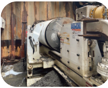
Drill rig advances the casing pipe as required based on formation resistance
