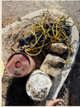
Debris pushed out from the medium density bare pig (left) included 5-gallon drums, an extension cord and grout
