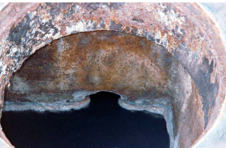
Figure 4: 6-yr evaluation - Hard surface with no corrosion; sparked when hit with a pick
