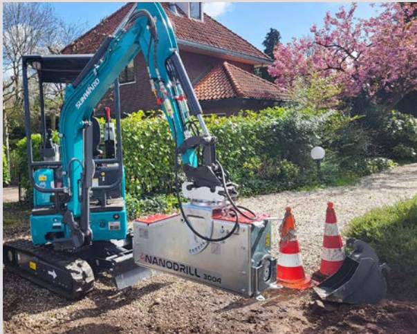
Ultra-compact, highly portable solution is designed to attach to a mini excavator
