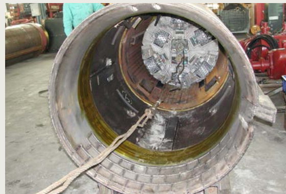
Shuttlemole TCSM recovery process
